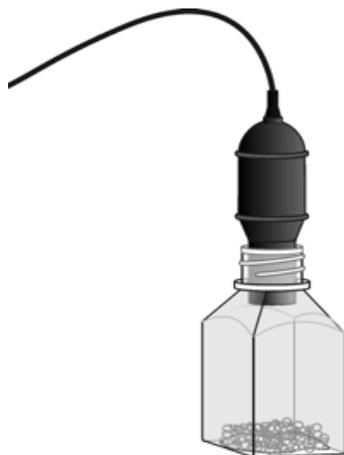
Figure 1. Vernier O<sub>2</sub> gas sensor probe and reaction chamber ready to collect data.
